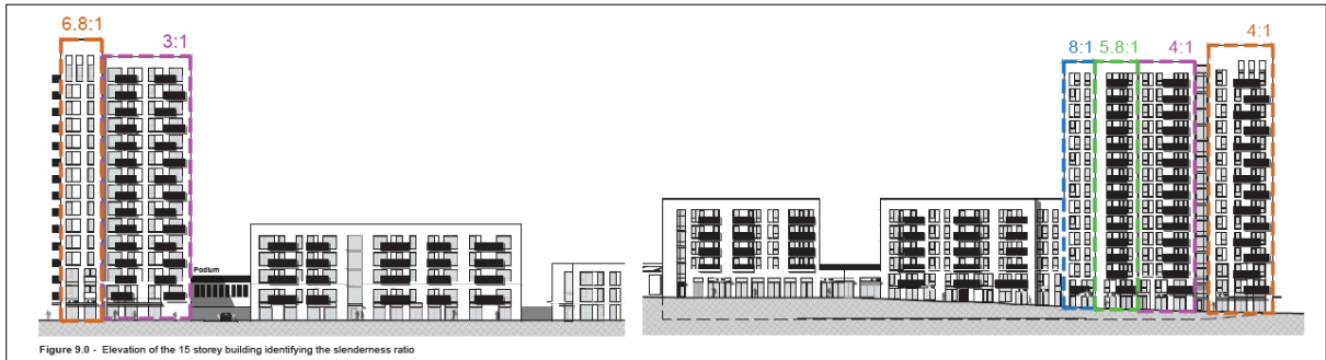
Figure 6.14 Elevation of the Landmark Building illustrating the Slenderness Ratio. (Source: Architectural Design Statement).
