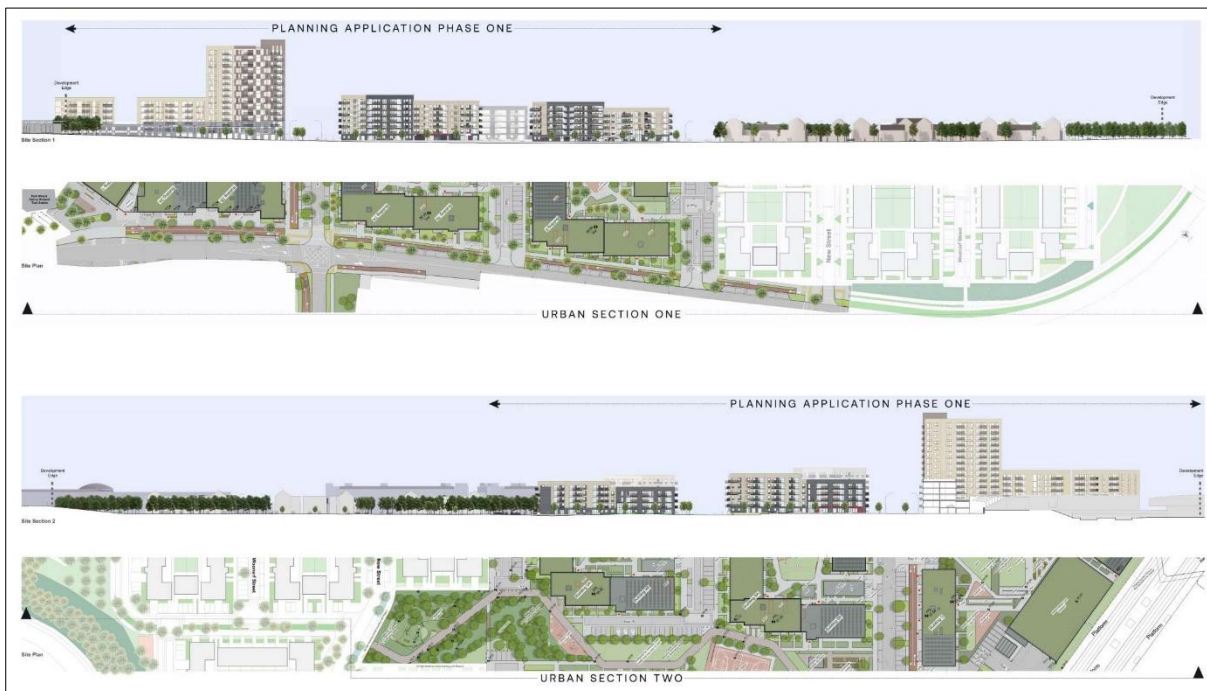
Figure 6.15 Contiguous Sections showing transition in height across the lands (Source: VDA / CCK Design Statement)
