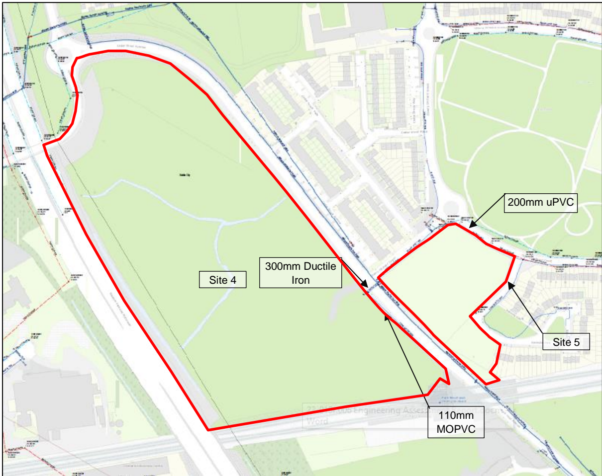
Figure 6.18: Irish Water Watermain Network Map Extract. (Source: Waterman Moylan)
