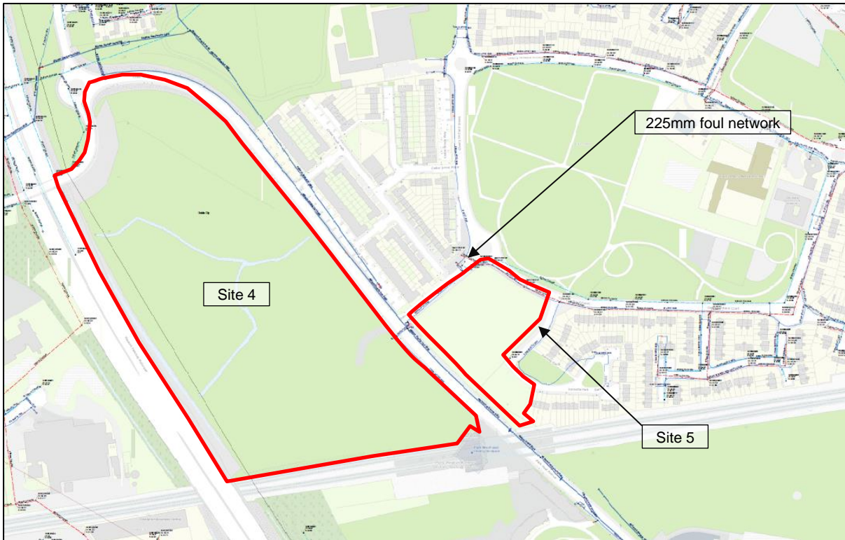
Figure 6.19: Foul Water Network Map Extract. (Source: Waterman Moylan)
